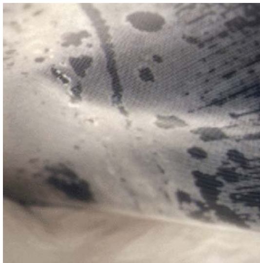
Fig. 1. Silica scale deposits on a RO membrane surface.
